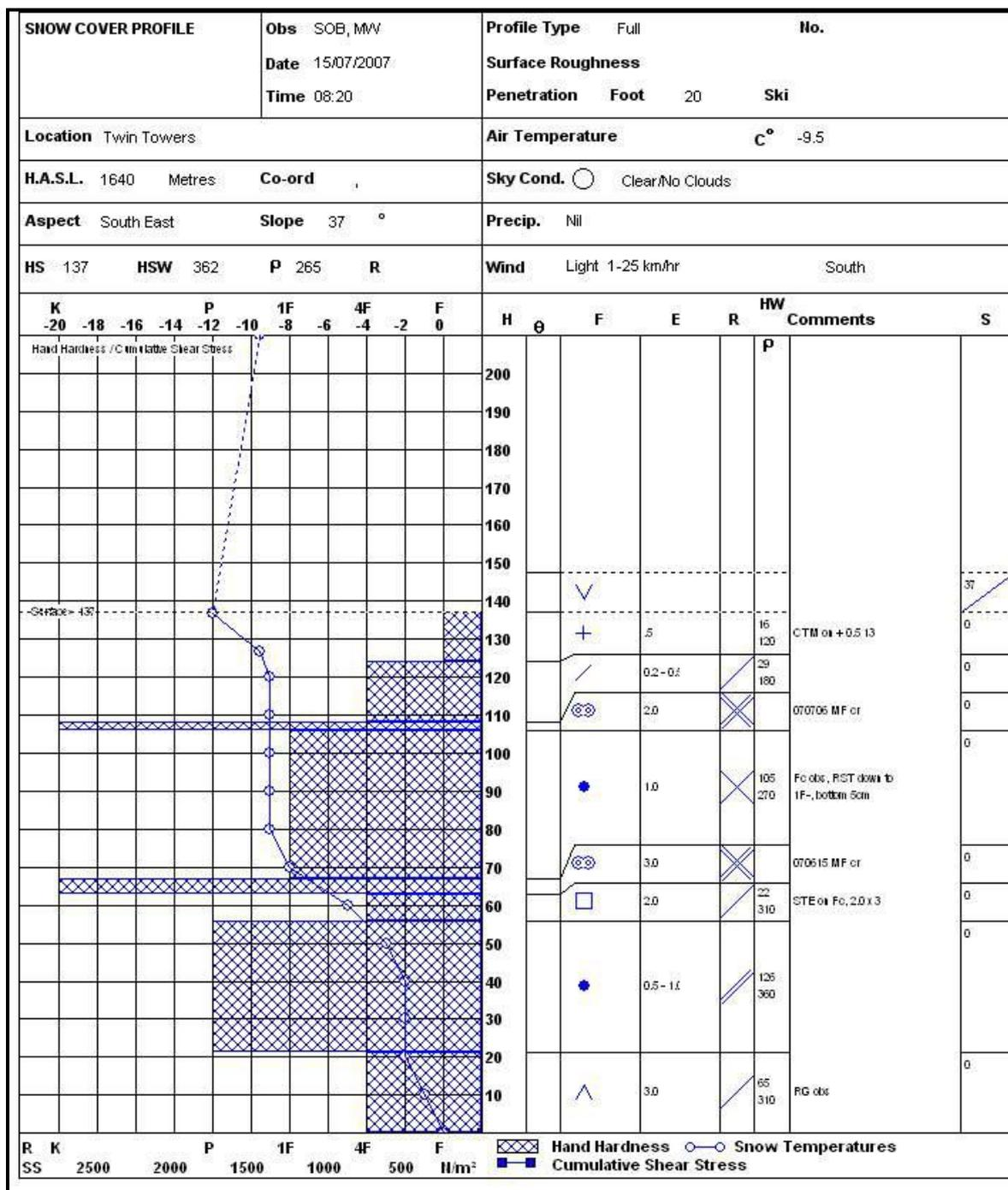
Figure 3: Graphical representation of a snow profile produced by the personal computer programme 'Snowpro 2006', Gasman Industries, Vancouver, B.C., Canada.
