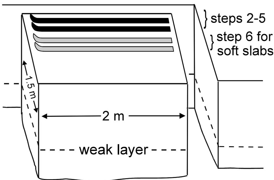
Figure 7: Rutschblock dimensions and ski/snowboard step positions
