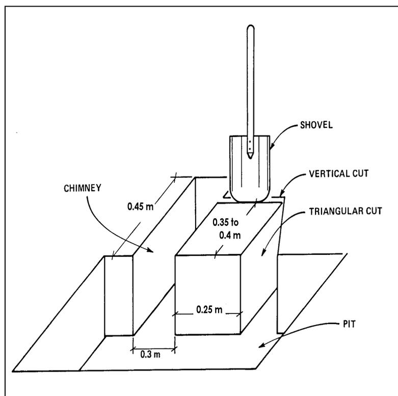
Figure 8: Shovel shear test snow column dimensions.
