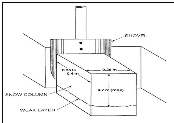
Figure 9: Shovel shear test application
