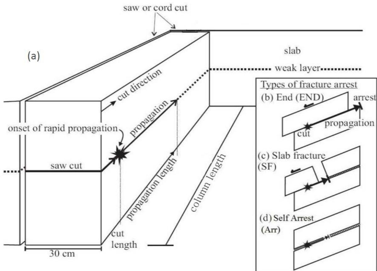
**Figure 12:** Schematic showing the PST column (a) and the observable results of propagation to end (b), slab fracture (c), and self arrest (d) (after Gauthier and Jamieson, 2007).
