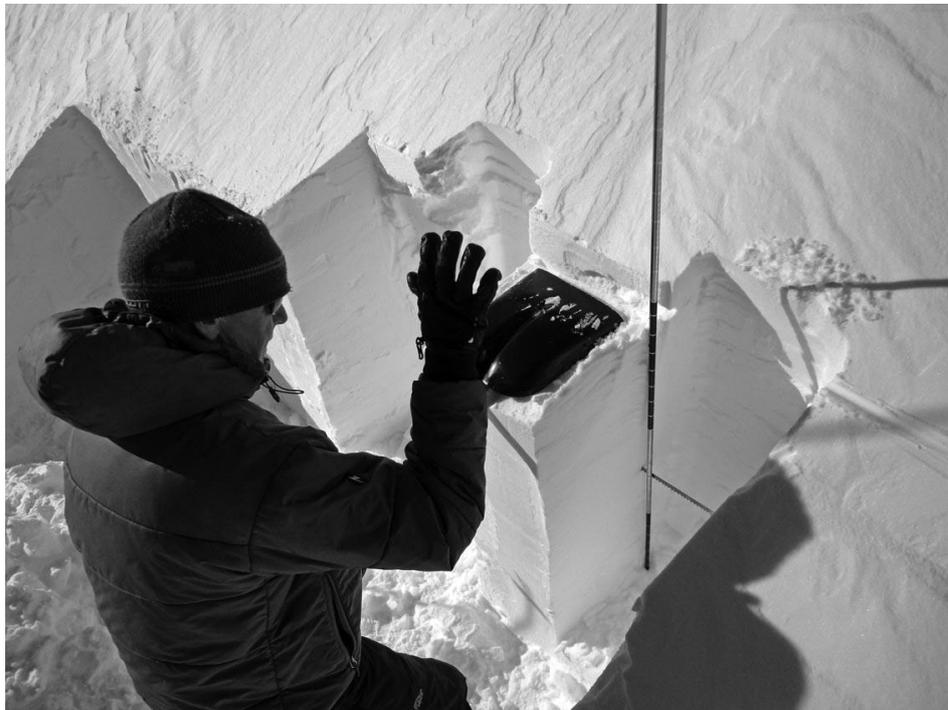
*Figure 10: Compression test technique and column dimensions.*
